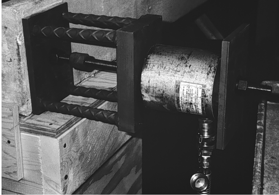
Figure A.16 Beam loading system.
