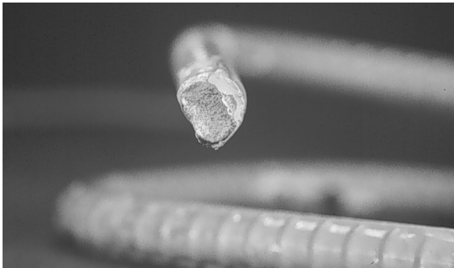
Figure 2.57 Patch at bar end of a stirrup hook that broke during autopsy (beam B23) after 4.3 years. Metallic surface beneath the patch was uncorroded.
