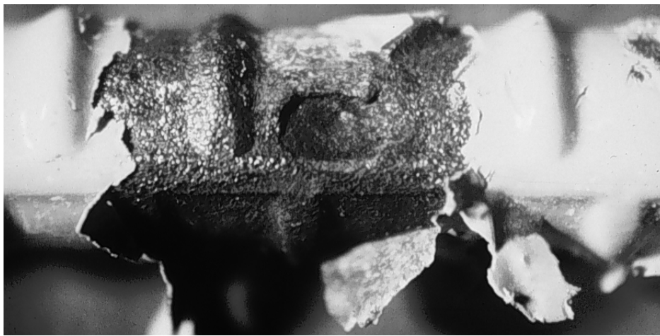
(b) Pitting on lower longitudinal bar
