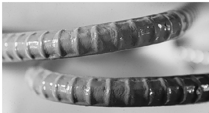
(b) As-received, patched condition of bends
