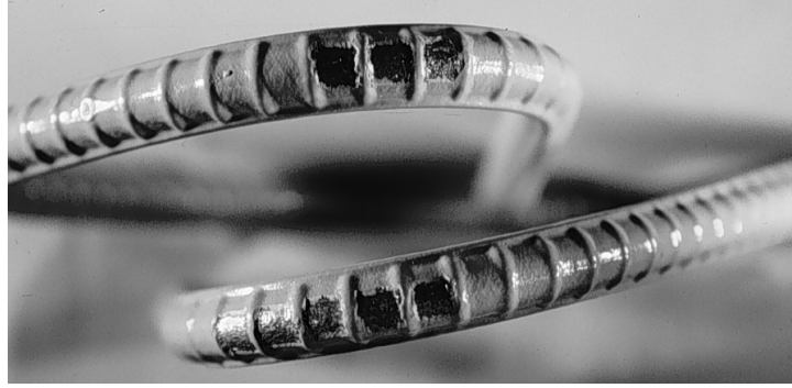
(a) 3% damaged bends
